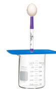
Figure 3. When flicked horizontally, the TupperWare lid knocks the marker out of the way, allowing the egg to land safely in the beaker of water.
