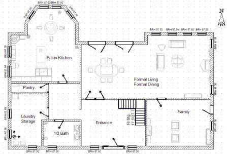
Floor plan: the most fundamental architectural diagram, a view from above showing the arrangement of spaces in building in the same way as a map, but showing the arrangement at a particular level of a building. Technically it is a horizontal section cut through a building, showing walls, windows and door openings and other features at that level. The plan view includes anything that could be seen below that level: the floor, stairs (but only up to the plan level), fittings and furniture.
