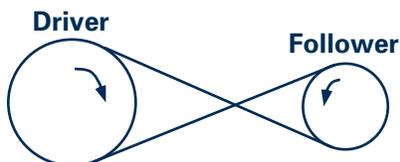
c. The magnitude of the effect is the same as for the model in Part a, but the follower turns in the opposite direction. Thus, the transmission factor could be  $-\frac{r_1}{r_2}$ , where the minus sign indicates that the wheels are turning in opposite directions. That difference is the only one necessary.
