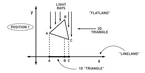
There is a source of light that is far enough away for its light rays to be parallel to the y-axis by the time they arrive at the triangle. We can think of the triangle's projection on the x-axis as the shadow that it casts. A one-dimensional being would experience this as an area of darkness. If we label the vertices of the triangle and allow it to be semi-transparent, then the "linelander" will also
