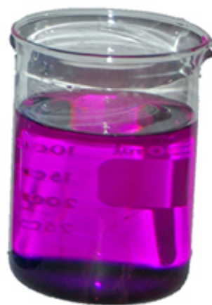
Potassium permanganate can oxidize many chemical compounds, which in turn reduces the manganese from its +7 oxidation state to a lower oxidation state. When this happens, the deep purple color disappears—a very noticeable indicator that a reaction has taken place. © Wikimedia Commons, Public Domain.
