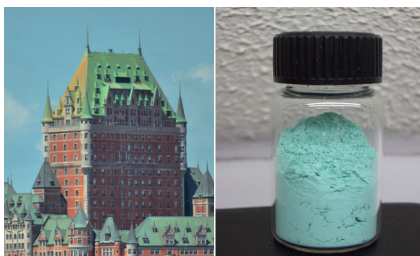
Figure 1-11. Copper Carbonate Forming on a Copper Roof; Pure Copper Carbonate in a Vial
