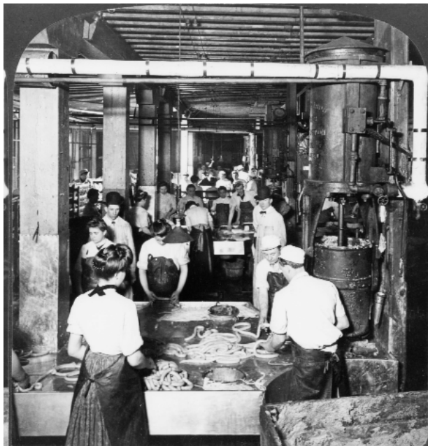
[7110] H. C. White Company, Making Link Sausages—Machines Stuff 10 Ft. per Second (c. 1905), courtesy of the Library of Congress [LC-USZ62-50217].
