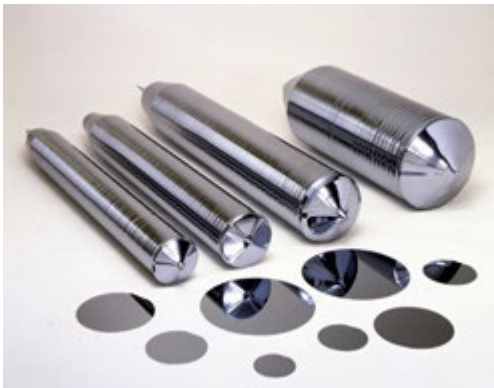
Figure 23.4: Silicon ingots and polished wafers.
