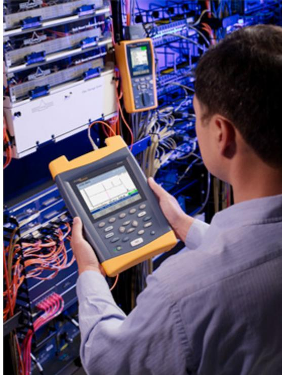
**Figure 4:** An optical time domain reflectometer in use.
