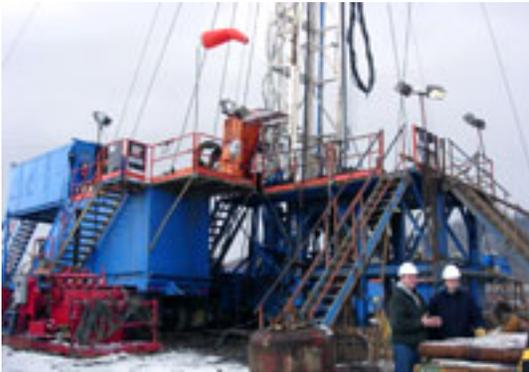
Drill rig for test site for sequestering carbon underground. Courtesy of Larry Hamill
