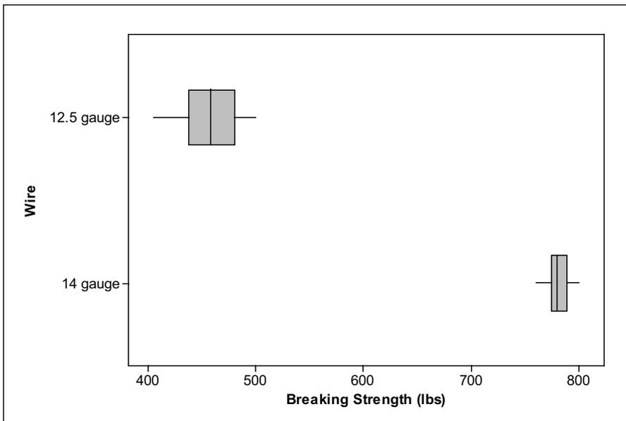
b. The mean breaking strength for the 12.5-gauge, low-carbon wire is 458 lbs. The mean breaking strength for the 14-gauge, high-tensile wire is 780.75 lbs. The 14-gauge wire has the larger mean breaking strength.
